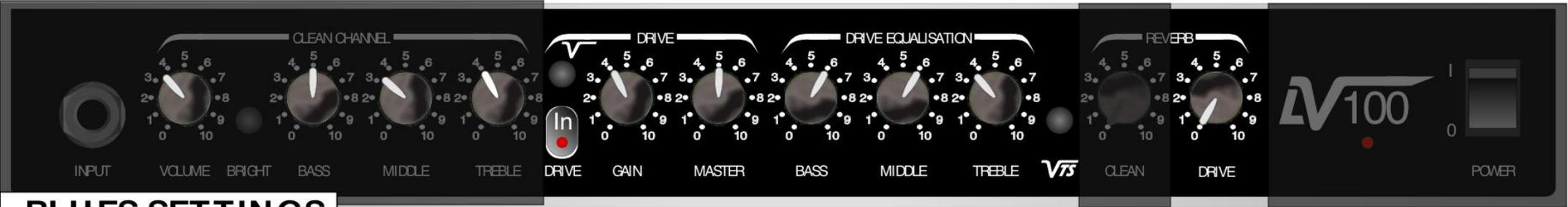
Blues Settings panel showing the following knob positions: INPUT (Off), VOLUME (5), BRIGHT (5), BASS (5), MIDDLE (5), TREBLE (5), DRIVE (In), GAIN (5), MASTER (5), BASS (5), MIDDLE (5), TREBLE (5), CLEAN (5), DRIVE (5), and POWER (Off). The 'CLEAN CHANNEL' label is positioned above the first four knobs, 'DRIVE' above the next two, 'DRIVE EQUALISATION' above the next three, and 'REVERB' above the last two. The 'VTS' logo is visible between the Drive and Reverb sections.
